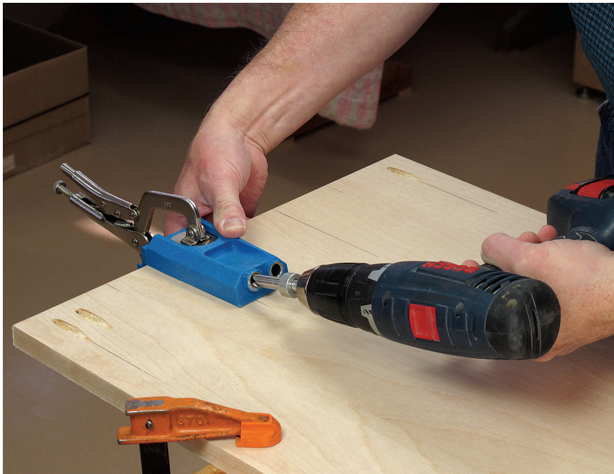
Drill the pocket screw holes using a pocket-hole jig. Bore two side-by-side holes at the front edges, as shown here, for increased holding power where it matters most.
