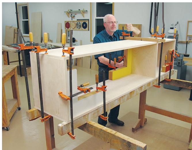
Glue and clamp the side cabinet pieces together, making sure the assemblies remain square when you tighten the clamps.
