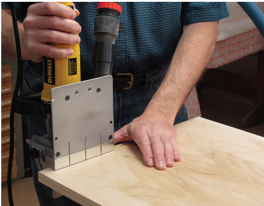
Cut the biscuit slots in the bed cabinet sides for joining the top, bottom and backs. The biscuits will keep the joints aligned when pocket screws are inserted.
