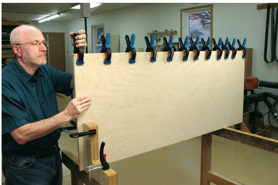
Glue and clamp the 1/8"-thick edging pieces to the edges of the upper and lower back panels. A bunch of Rockler medium-size Bandy Clamps makes quick work of this task. Push them down as hard as you can to apply maximum pressure for tight glue joints.
