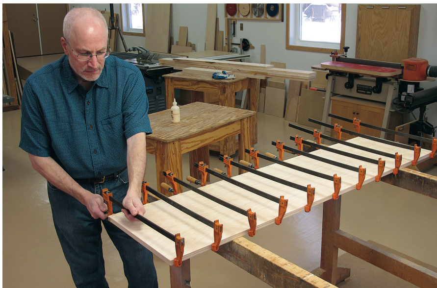
Glue and clamp the 3/4"-thick edging pieces to the bed cabinet plywood. Place bar clamps at 6" intervals. Clean up wet glue squeeze-out with a rag, and scrape the rest away after it has cured.
